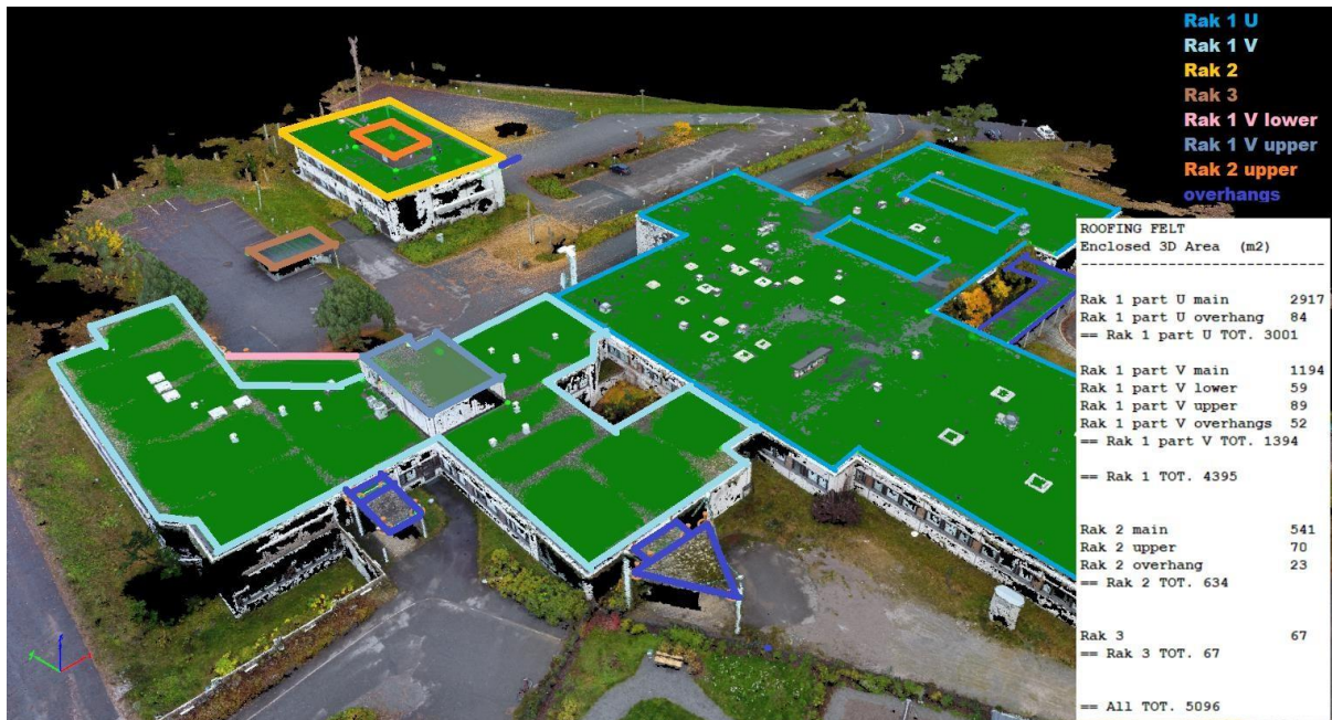
Image 13 - Calculating the amount of roofing felt from the point cloud. Note: coloured markings are hand-drawn and added for the sake of clearance. (Image: Esa Hannus.)
