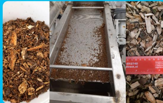
In Mikkeli, bio-waste pre-treatment involved three steps. Bio-waste was crushed for size reduction, ensuring efficient reactor space use. Material streams were mixed for uniformity,
