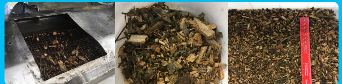
In the city of Apeldoorn, an unconventional biochar-based treatment system has been implemented for rainwater. This system functions as a pre-soil adoption filtration method, effectively purifying the water before it permeates into the soil. Although the demonstration is currently in progress, conclusive results have not yet been attained for dissemination.
