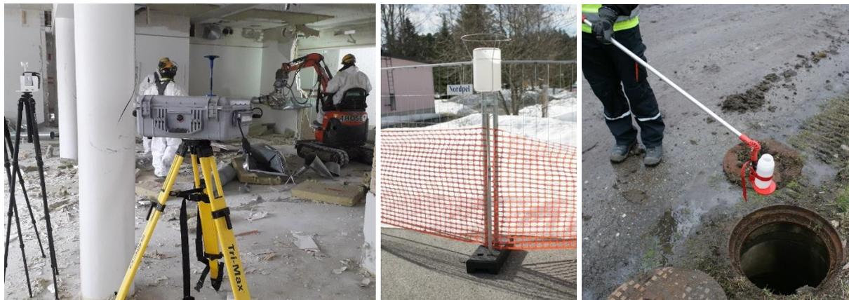
*Figure 5. Real-time dust monitoring with DustTrak Aerosol Monitor during the internal demolition phase in Pankalampi demolition site (left), dust deposition collectors (middle) and water sampling (right) in Pankalampi demolition site (photos Juha Vihavainen).*
