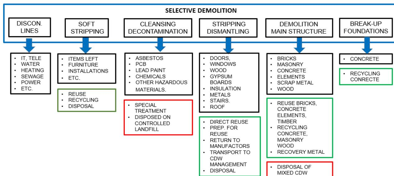
Figure 14. Phases of selective demolition (Lauritzen 2022)
