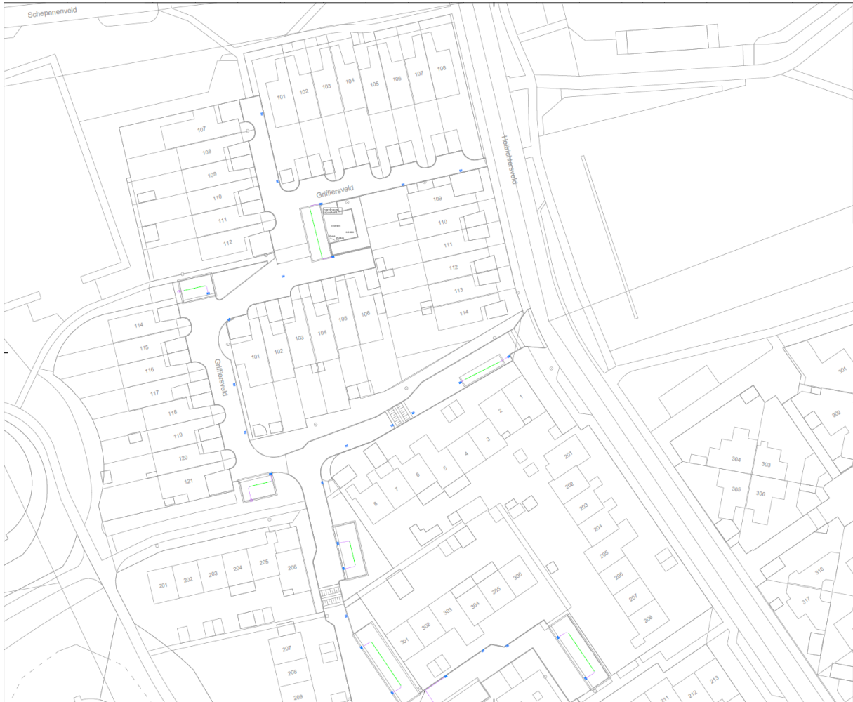
Figure B.3: A revision drawing that shows in green the actual location of the storm water infiltration system under beneath the road after renovation took place.
