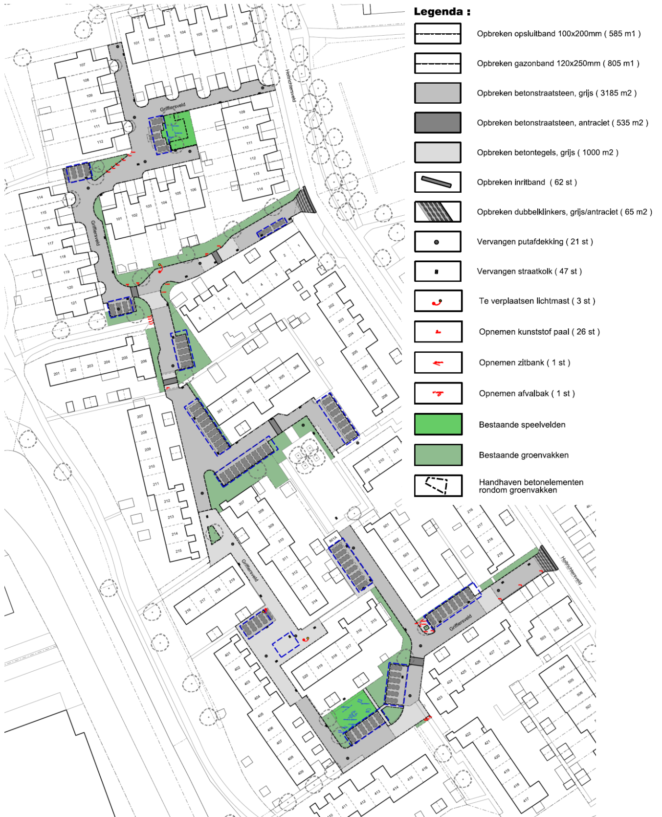
Figure B.2: Drawing showing which elements need to be taken out of the road and might come available for reuse.
