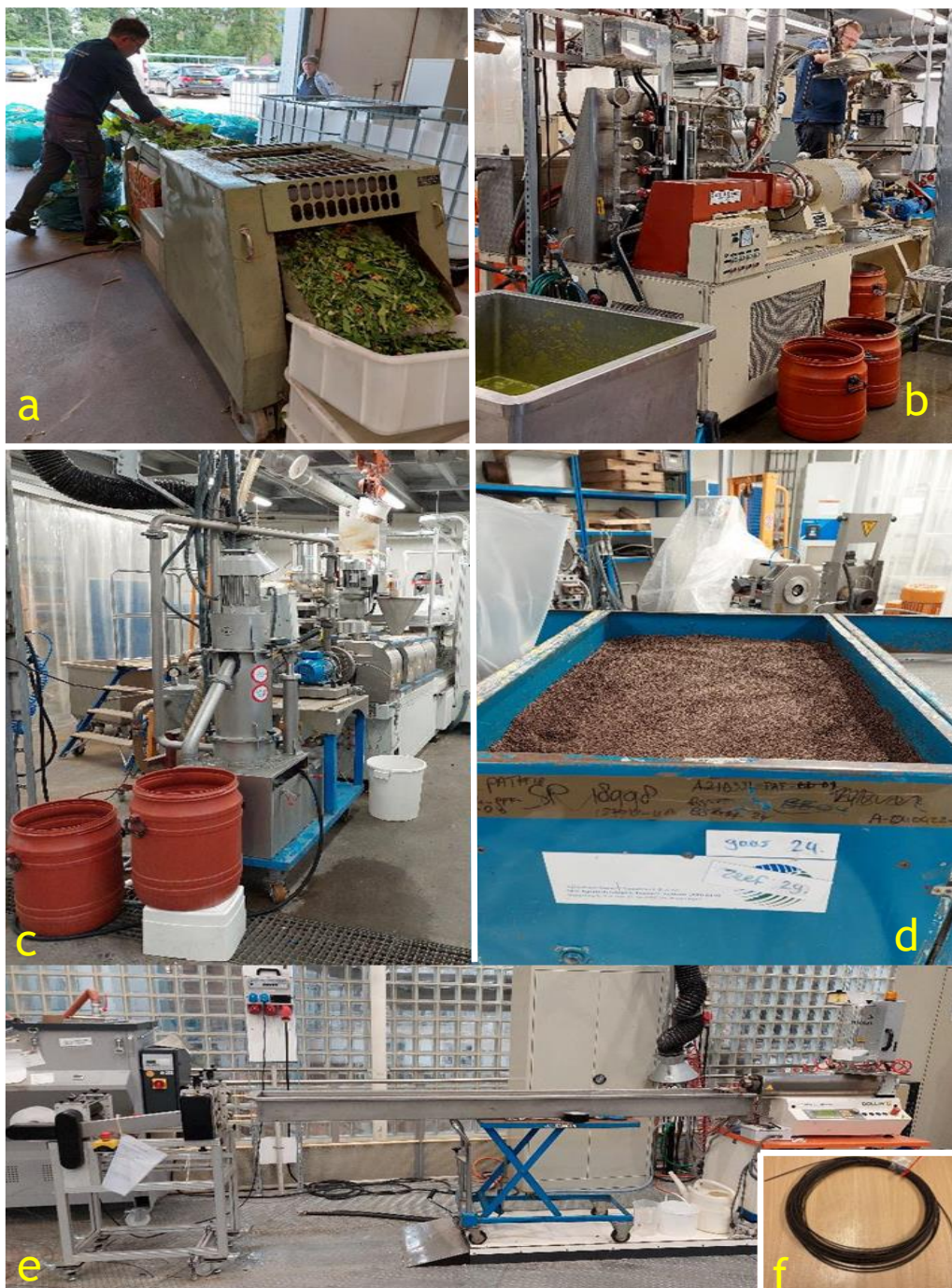
Figure 47: The demo-processing of JK to filament (a. Cutting the JK to reduce stalk length, b. Mechanical extraction of fibres using a disk refiner, c. Compounding and pelletising PLA and JK, d. Drying of the pellets, e. Filament production, f. dried filament.
