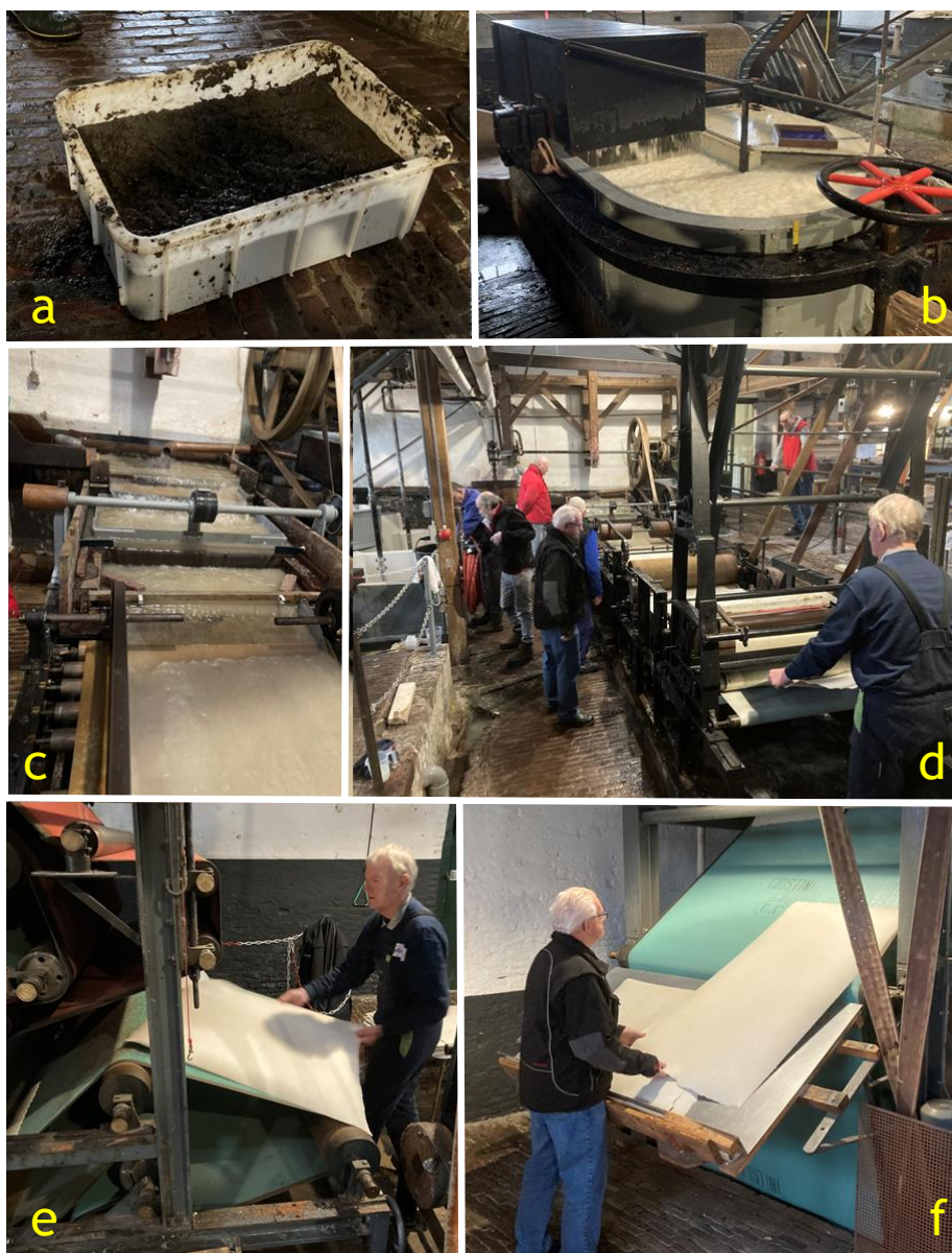
Figure 41: Paper production at De Middelste molen (a. part of the grass pulp, b. Valley beater, c. sieve section of wet end, d. press section of wet end, e. transfer by hand to drying section, f. dried paper coming from the drying section)
