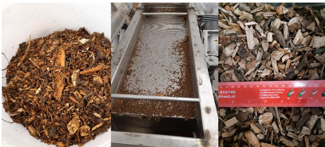
Figure 26 Vibration screening at WFBR (Left, chipped pruning, middle vibration screen, right, desired fraction)
