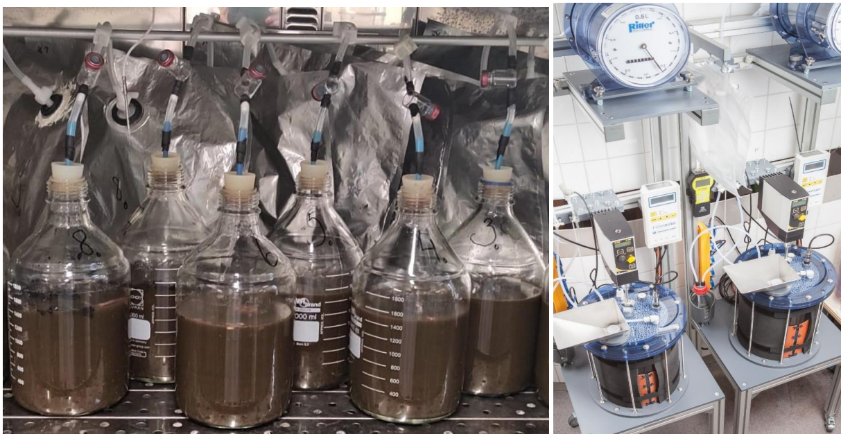
Figure 13. 2 L bottle batch reactors and 15 L pilot scale reactors were used in the demonstration experiments to optimise dry fermentation process of bio-waste (photos Tiina Saario (left) and Manu Eloaho (right)).
