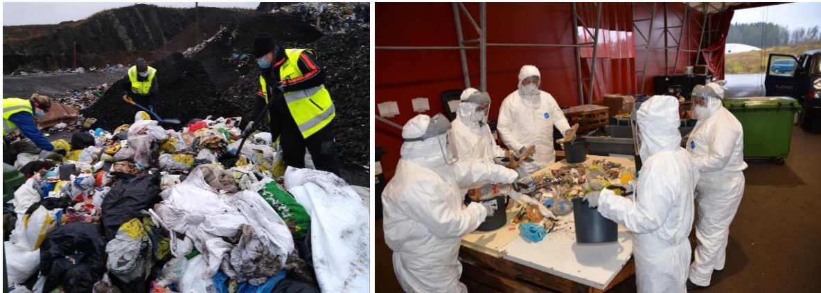
Figure 8. Composition study was performed to find out the share of recyclable bio-waste in household mixed waste of Peitsari area before and after demonstration actions. Left: sampling. Right: manual sorting of mixed waste. (Photos Hanne Soininen and Anne Laitinen).
