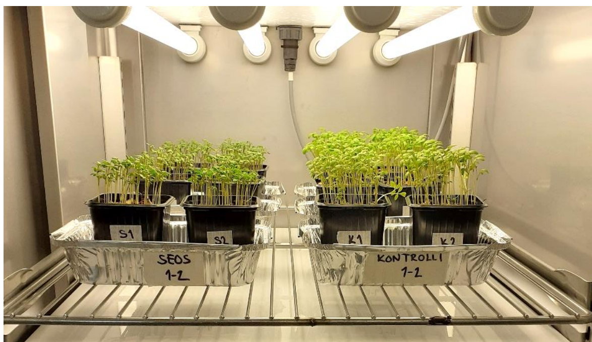
Figure 18. Plant growth tests were performed for soil improvement product and pelletised granules produced from bio-waste-based digestate of biogas plant (photo Janne Junninen).
