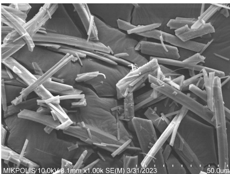
Figure 16. A scanning electron microscope (SEM) picture from struvite precipitate recovered with electrochemical method from liquid fraction of biowaste digestate. (Picture Xamk, Mikpolis laboratory)
