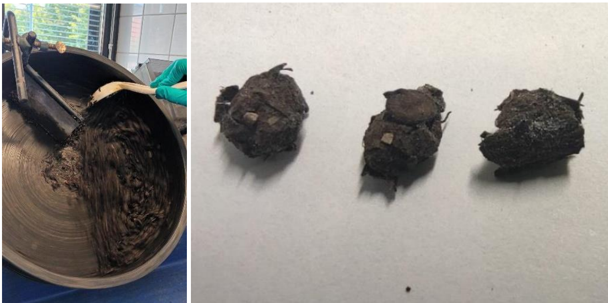
Figure 17. Pelletising of the dry fraction of bio-waste-based digestate of biogas plant was demonstrated to produce granules for fertiliser use. (Photos Tiina Saario)
