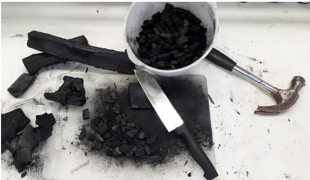
Figure 14. Birch-based biochar from local company was tested as an additive component to enhance biogas process (photo Tiina Saario).
