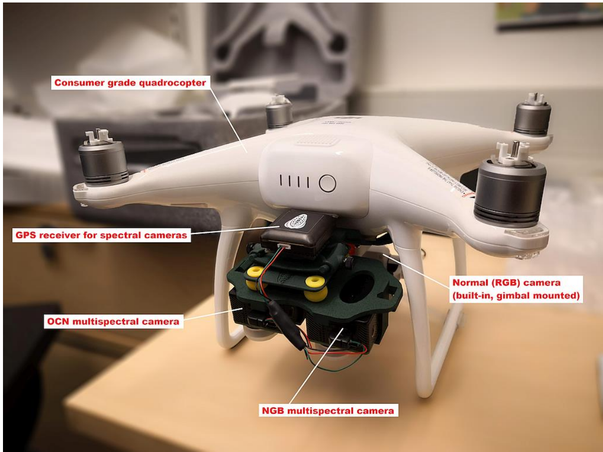
Image 2 - A consumer grade quadcopter equipped with two multispectral cameras (image: Esa Hannus).
