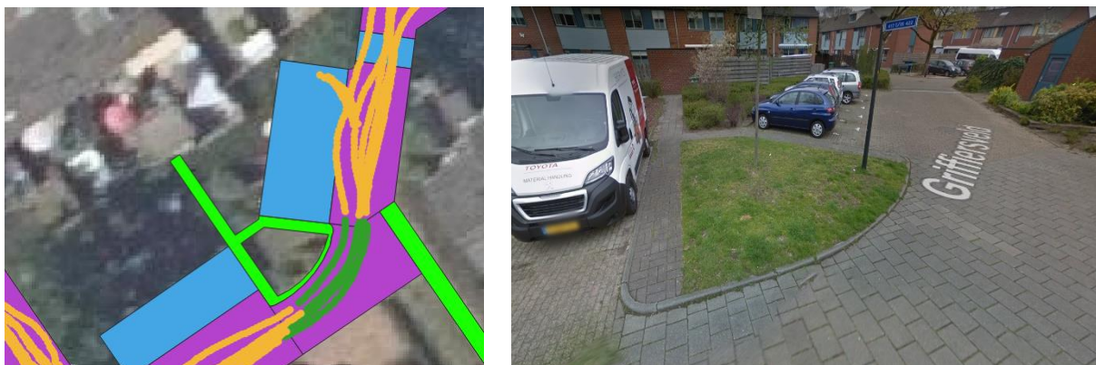
Figure 5. Although the purple surfaces indicated no change in pavement in the asset management system; the colour difference in the scanning routes did give the indication that different sorts of pavement were applied, namely concrete pavers and tiles (by courtesy of Pieter Ausema).
