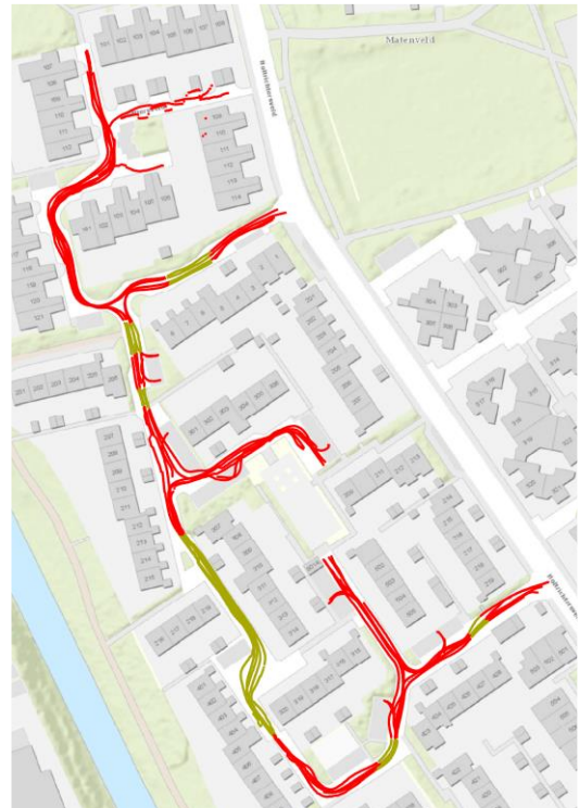
Figure 4.16. Applied pavement materials (red = concrete pavers, green = concrete paving slabs).
