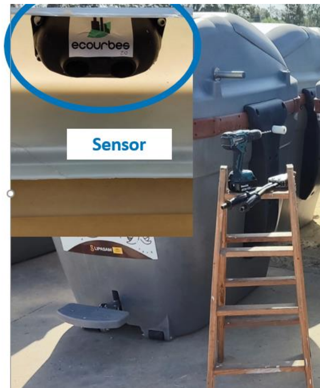
Figure 18. Detail of level sensor installed in a container from Seville CityLoops route.
