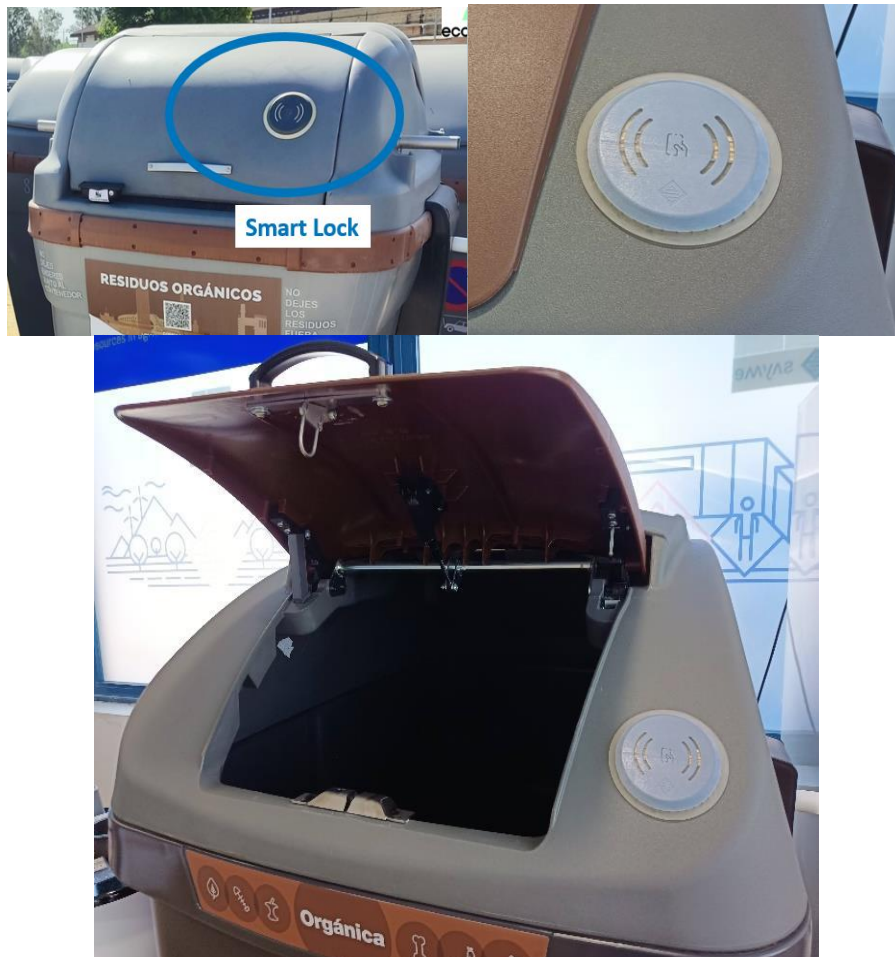
Figure 15. Details of Smart lock collection system installed for CityLoops collection route.
