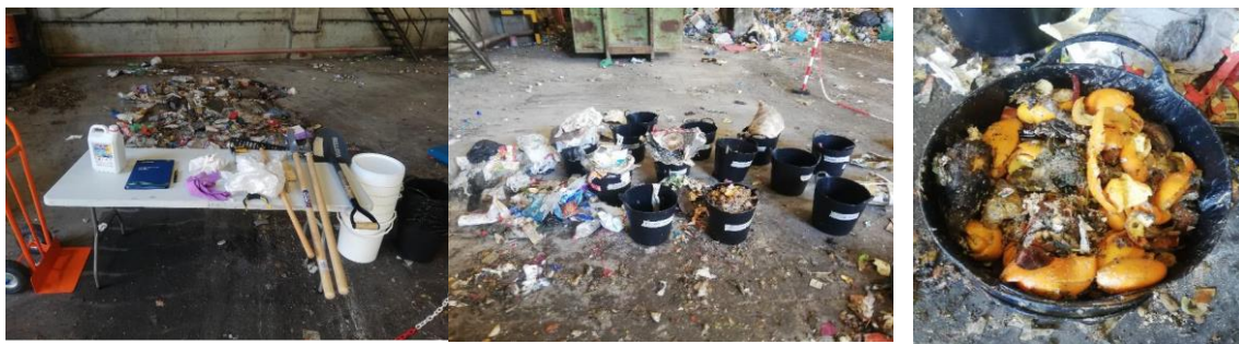
Figure 33. Pictures taken during one of the physical characterizations carried out. Worktable, buckets with separated waste and bio-waste sample.
